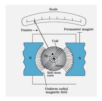
Principle: When a current carrying coil is kept in a magnetic field, it experiences a torque.
